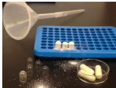
Figure 1. Modified pipette tip and rack for filling capsules with bean flour.
