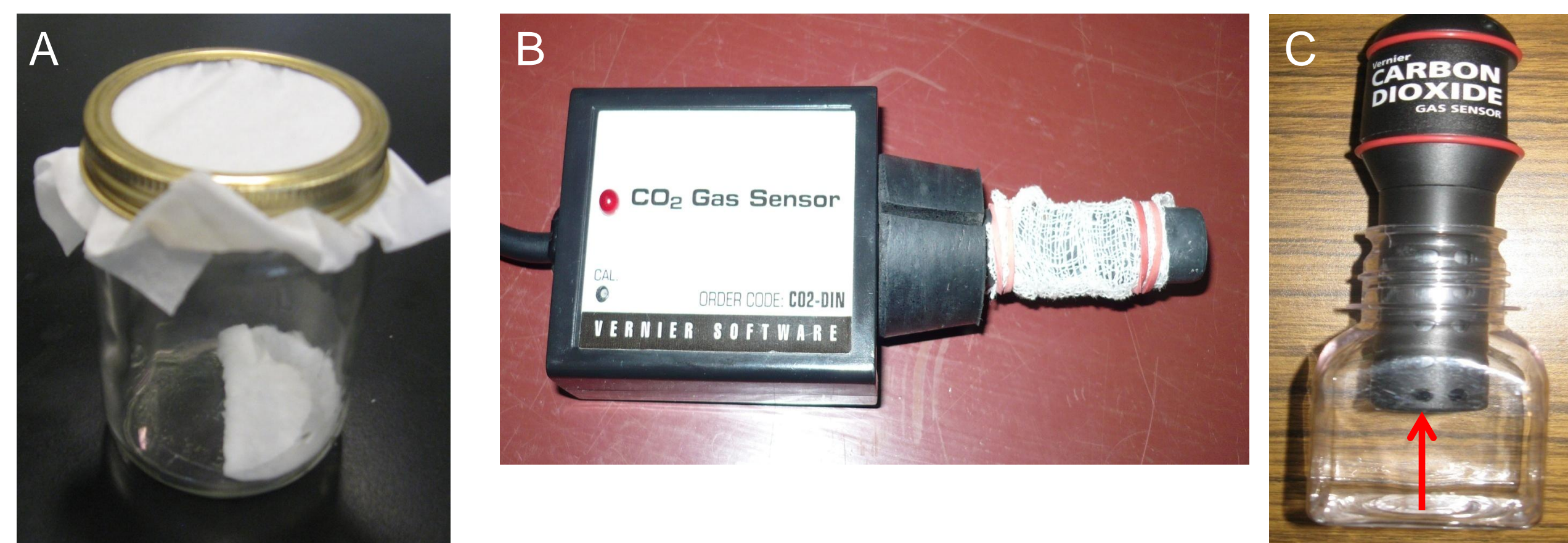
Figure 3. Representative equipment. A) Feeding chamber consisting of a small canning jar (pint) and Kimwipe lid. Cotton pad was saturated with nutrient solution and placed in jar prior to introduction of 25 adult beetles. B and C) Two different styles of Vernier Carbon Dioxide probes used for metabolic assessment. Gas ports (indicated by red arrow in C) were covered with cheesecloth (shown in B) prior to insertion in collection chamber. We used 50ml Falcon tubes and 125ml Nalgene bottles (shown in C). The set up for oxygen detection was similar.
