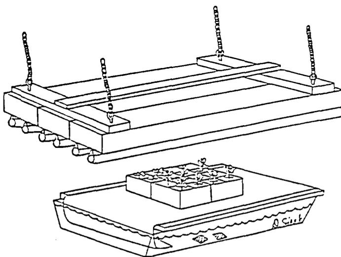
Figure 1. Light bank and watering system.
