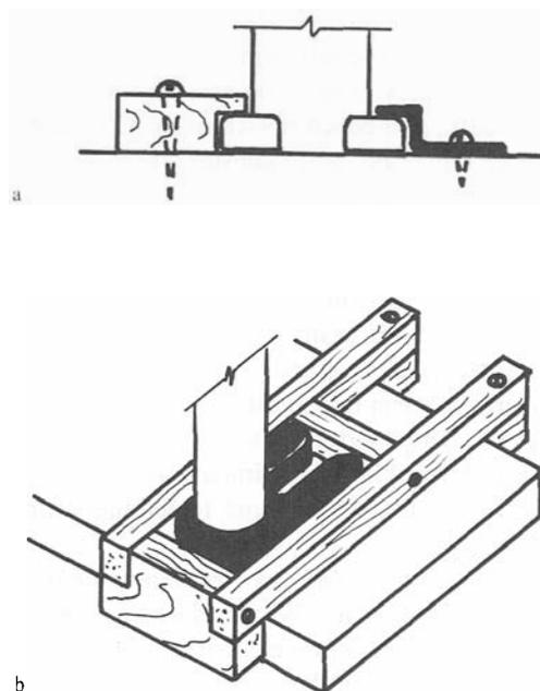
**Figure 1.5.** Two types of microscope braces devised by Roy Tombaugh. (a) Wooden or metal offset bar clamps which screw into the table top. (b) A wooden frame which hooks over the table top to prevent lateral movement of the microscope.
