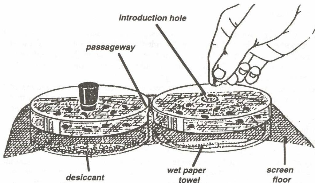
**Figure 1.4.** Apparatus for studying the orientation of isopods, set up to study humidity preference in constant light.
