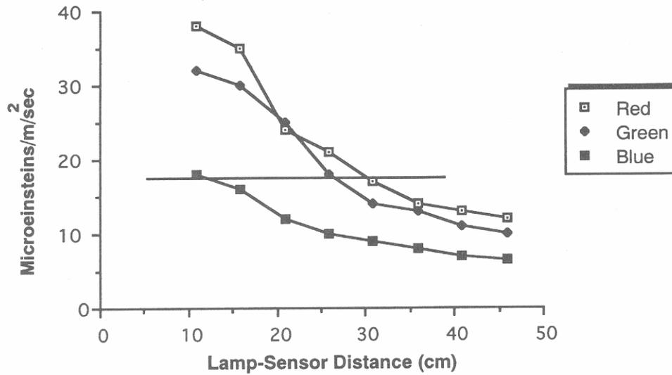
**Figure 1.6.** Relationship between light intensity ( $\mu\text{E m}^{-2} \text{sec}^{-1}$ ) and the lamp-bulb distance (cm), using 150-watt incandescent and two 25-watt fluorescent bulbs as a light source, for three filters (one sheet Dark Urban Blue, #866; one sheet Medium Green, #874; and three sheets Medium Red, #823). Light intensity was measured with a Li-Cor model LI-185A quantum/radiometer/photometer.
