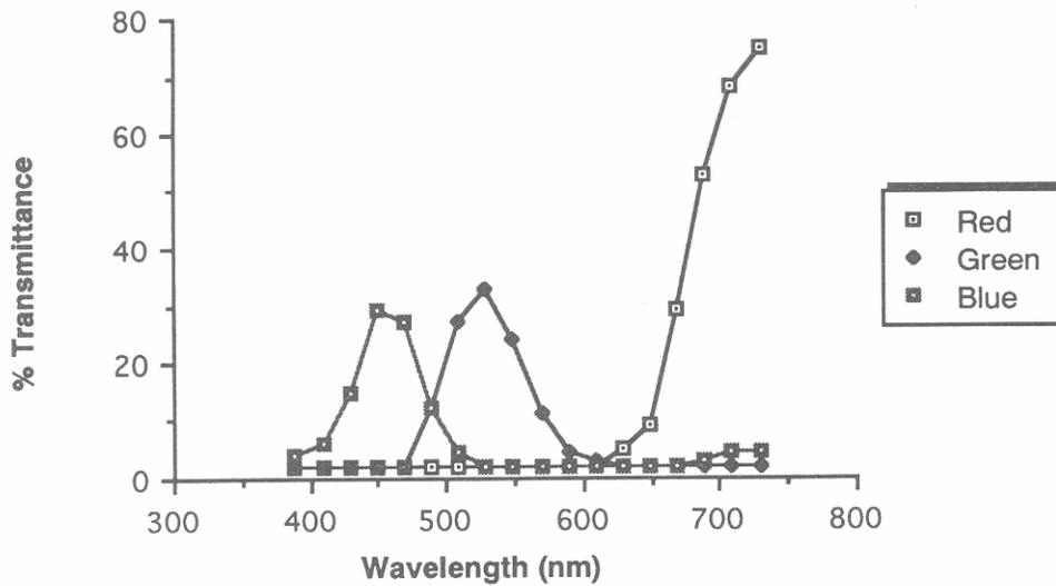
**Figure 1.7.** Transmission spectra for three filters (one sheet Dark Urban Blue, #866; one sheet Medium Green, #874; and two sheets Medium Red, #823) obtained with a Spectronic 20 spectrophotometer.
