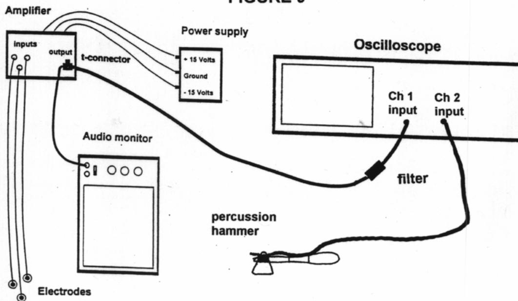
2. Set the oscilloscope sweep speed (**SEC/DIV**) to 10 msec/div. Press **CH2/MENU** button until a second trace for Channel 2 is seen on the oscilloscope screen. Adjust **Ch2 POSITION**, if needed.
