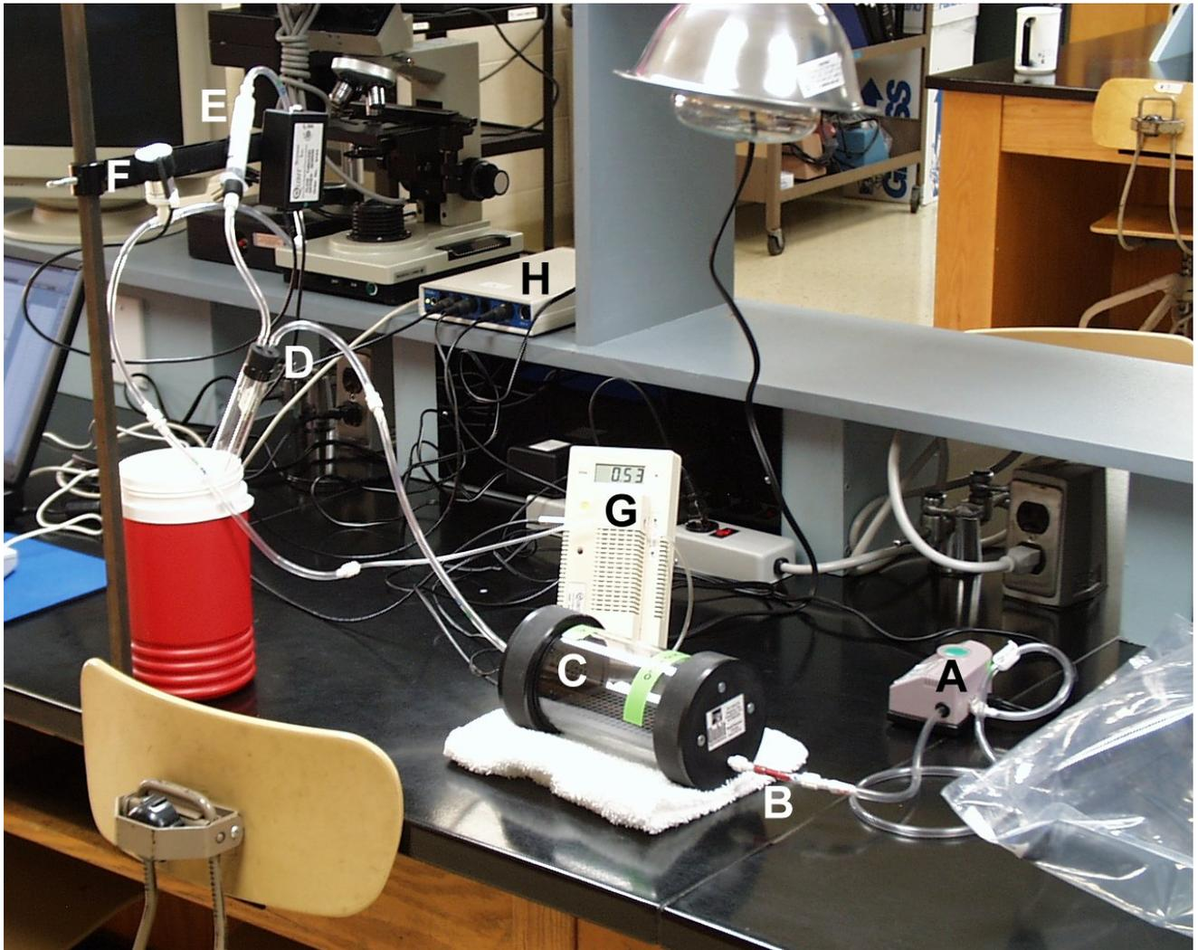
**Figure 2.** Photograph of setup for animal respiration study showing components in the order of gas flow.
