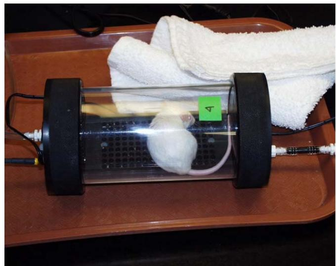
**Figure 5.** Large size animal cuvette. Suitable for mouse and similar size animals. The enclosed air is stirred by an electric fan.
