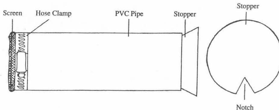
**Figure 14.3.** Rat restraint device.
