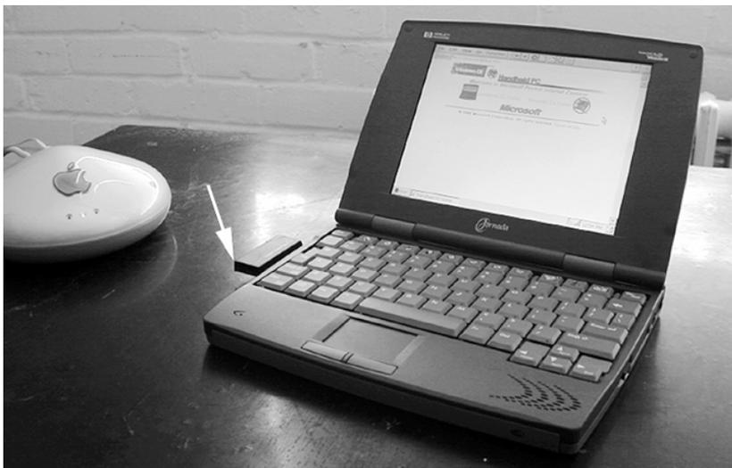
**Figure 1.** The Jornada 820 computer and Apple Airport. The Jornada 820 is a mini-laptop computer with a large screen and a keyboard. It can access the internet via a wireless networking card (arrow) when a base station (the Airport) is connected to an ethernet port.
