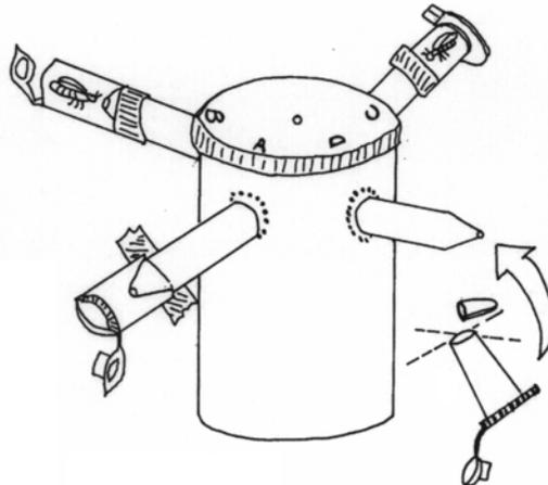
**Figure 19.3.** This bioassay chamber uses four microcentrifuge tubes as replaceable housing for the experimental subjects and substances. Nonwoven polyester caps separate the interior of each tube from the interior of the bioassay chamber. These barriers allow odors and sounds to pass through, but *Melittobia* will remain separated — unless, as occasionally happens, a determined individual chews a hole through it!
