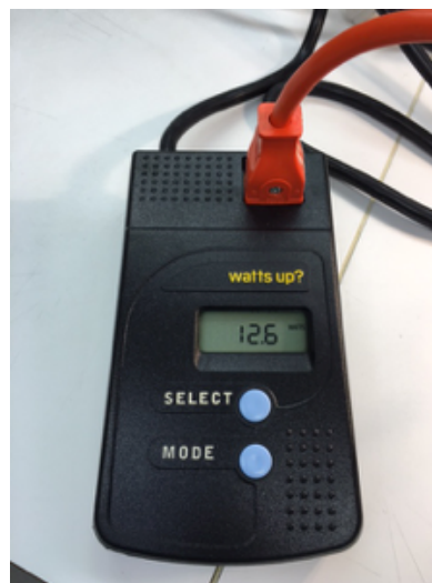
Figure 3. WattsUp Meter. This device measures the instantaneous power (watts) use of any 120v device plugged into its outlet (15A current or less). The WattsUp meter must be plugged into a 120v power supply, ideally, in this application, a switch controlled power strip.
