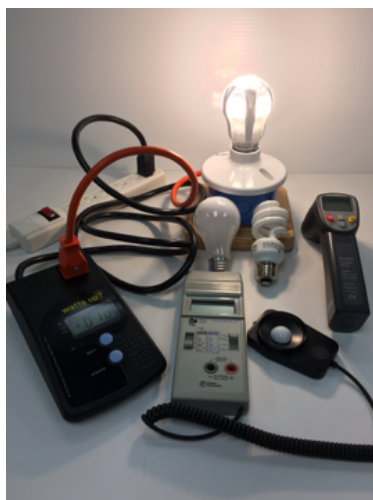
Figure 1. Light bulb fixture with measurement devices. Each of three light bulb types may be evaluated individually using a WattsUp meter (black unit on left), light meter (center) and laser thermometer (right).
