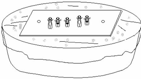
**Figure 4.** Use of saran wrap over the top of the ice to allow rescue of flies that fall off the metal plate. This method requires that the plate is pushed down well into the ice so that no air pocket forms between the saran wrap and ice or saran wrap and plate. If there is any space, the plate does warm and flies start to walk around.
