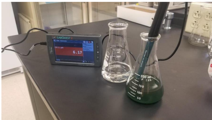
Figure 1. Two Erlenmeyer flasks: one control and one with Spirulina sp. pH meter probe inserted.
