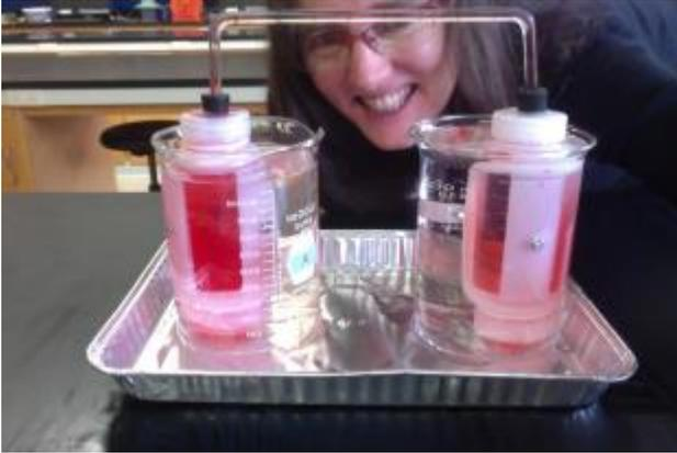
**Figure 2.** A pressure flow model built by students at Whitman College. The source cell (Cell A) is on the left. Note the water level in the two beakers. Pressure from the source cell has already caused the right beaker, with Artificial Cell B, to overflow.
