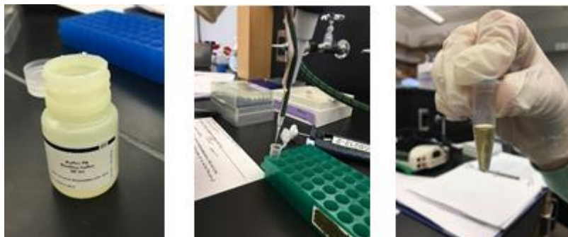
Figure 5. Buffer PB (left) gets added to the reaction (middle) and the solution should turn yellow (right)
