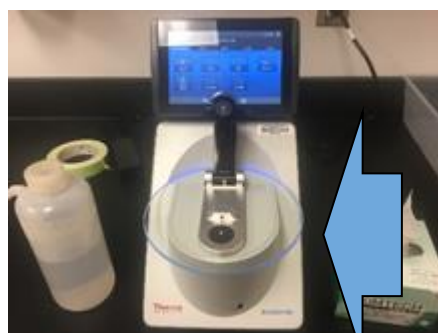
Figure 10. Arrow indicates where sample should be added to Nanodrop™
