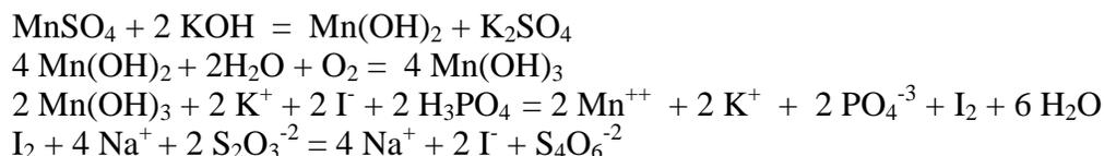
Winkler determinations are done routinely in testing water samples. We are using a modification called the Micro-Winkler that requires only 10 mL of sample (Burke, 1962). Take at least two samples every time you determine the DO.
