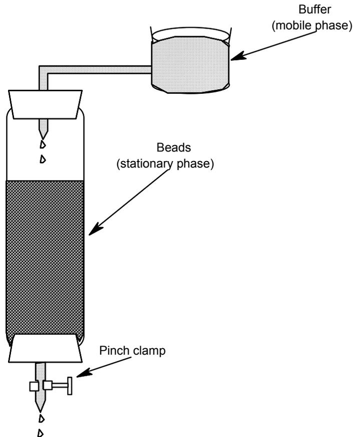
**Figure 3.2.** A simple column for ion exchange chromatography.
