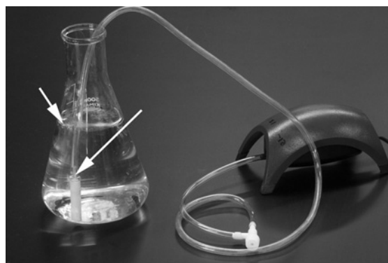
Figure 1. Simulated pond setup. Aeration is crucial to success, but keep bubbling to a minimum so that only a small portion of the surface (see arrows) is disturbed.
