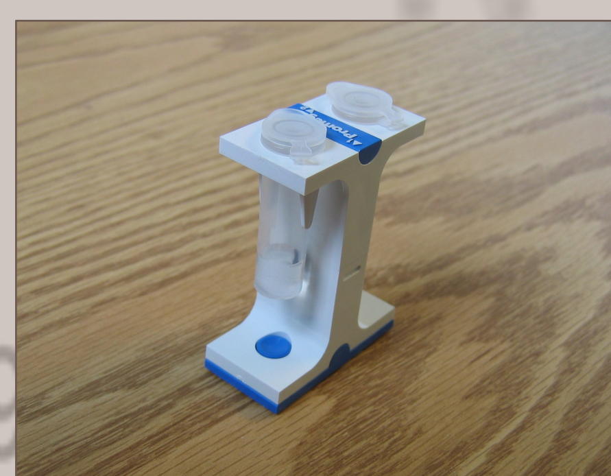
Figure 1. A magnetic stand with sample containing magnetic beads.
