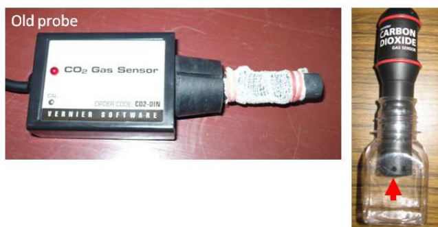
Figure 2. Gas sensors used in the described experiment were covered with cheesecloth or Kimwipes to prevent beetles from entering gas ports (noted by red arrow).
