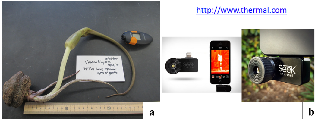
Figure 4. Methods of recording temperature changes in voodoo lily. a. Radio shack IR thermometer with voodoo lily bloom at Day 1. b. Seek Thermal camera and website.
