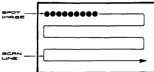
Sample scanning pattern of electron beam.
