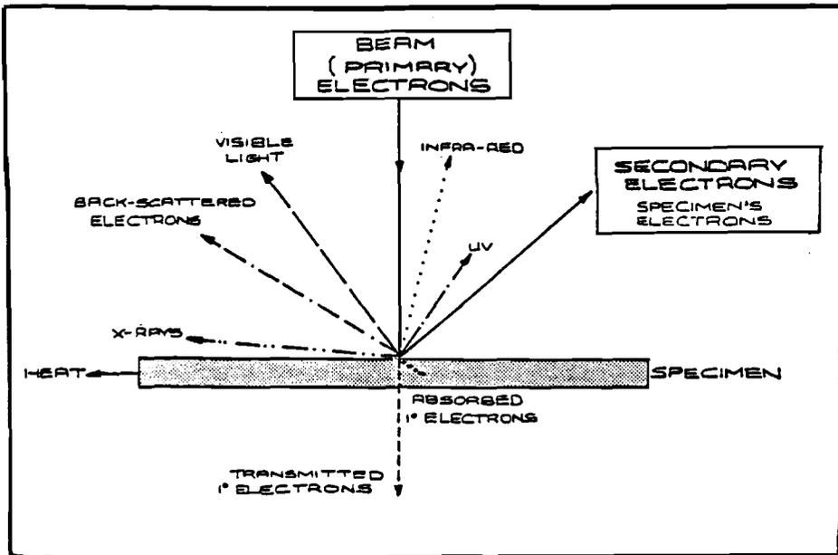
Effects of electron beam bombardment of a specimen.
