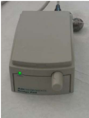
Figure 1: Bridge Pod to be used with hardware and software for the ADI force transducers.
