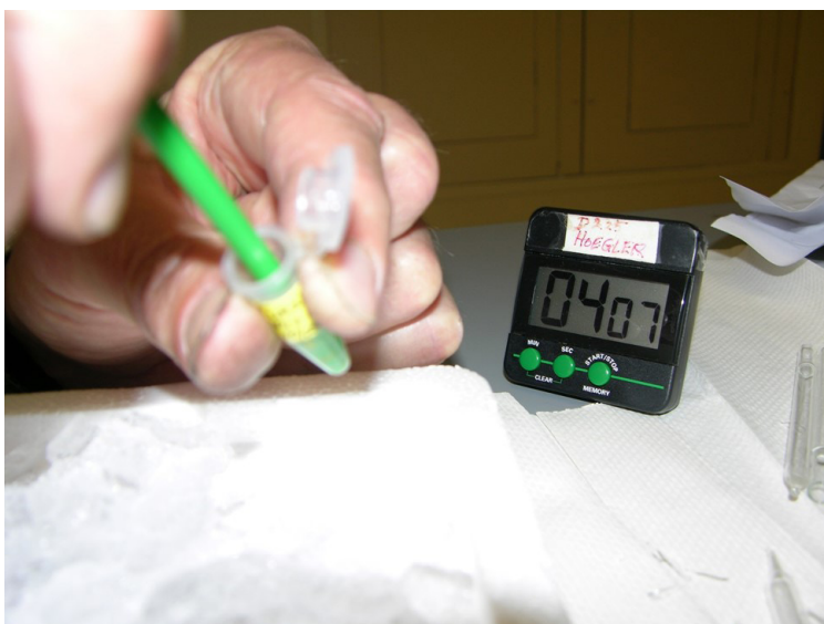
Figure 2. Seedling preparation procedure showing the use of plastic pestle to grind thawed seedlings within the microfuge tube.
