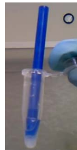
Hand-held pestle for grinding glass
