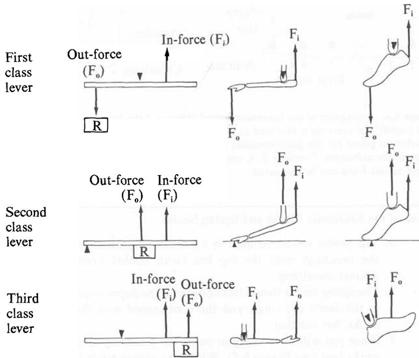
**Figure 6.3.** Illustration of three classes of levers as found in the movements of the arm and foot. R represents the resistance, against which the out-force is applied and the fulcrum is at ▲. (Adapted from M. Hildebrand: Analysis of Vertebrate Structure. Copyright © 1974 by John Wiley and Sons, New York. Reprinted with permission.)
