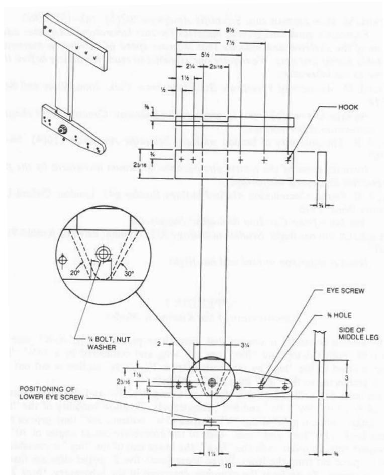
Figure 6.9. Plans for construction of the kinematic model.
