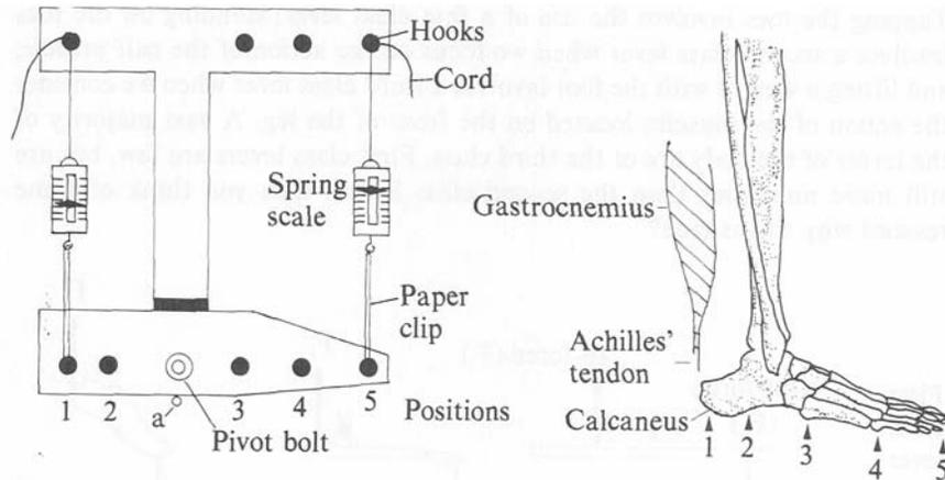
**Figure 6.4.** A diagram of the kinematic model (left) and the human lower leg and foot (right). An eye-ring is attached at position "a". Positions 1 and 2 represent attachment points for the gastrocnemius muscle, whose contraction produces an in-force on the calcaneus. Positions 3, 4, and 5 represent points on the front of the foot where an out-force can be measured.
