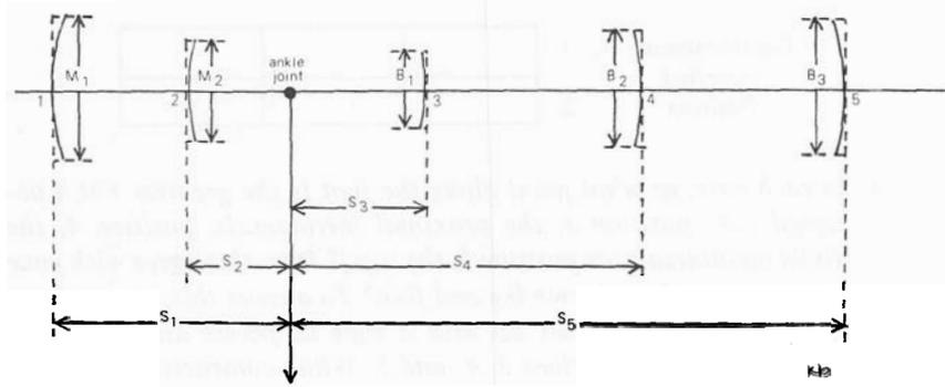
**Figure 6.8.** Diagram showing the relationship between the lever arms ( $S_1$ - $S_5$ ) at various position (1—5) in a simple lever system, and the distance of muscle contraction ( $M_1$ - $M_2$ ) and bone movement ( $B_1$ ,  $B_2$ ,  $B_3$ ) at these positions.
