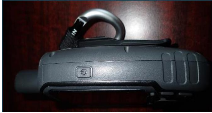
Figure 2: location of the power button on the Garmin 62sc unit
