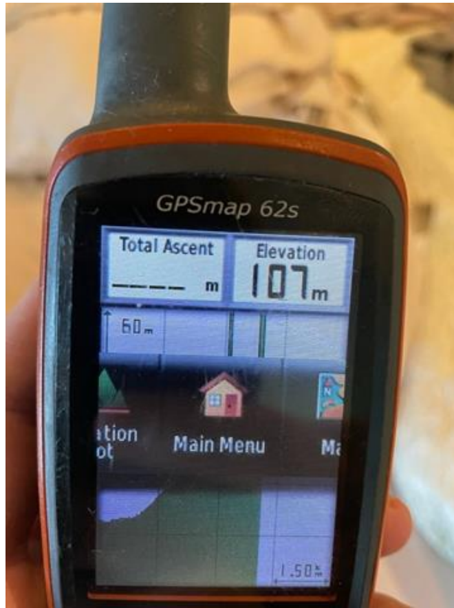
Figure 3: Navigating through the different pages of the Garmin 62sc unit - keep pressing the “page” button until you get to the Main Menu (shown in the figure).
