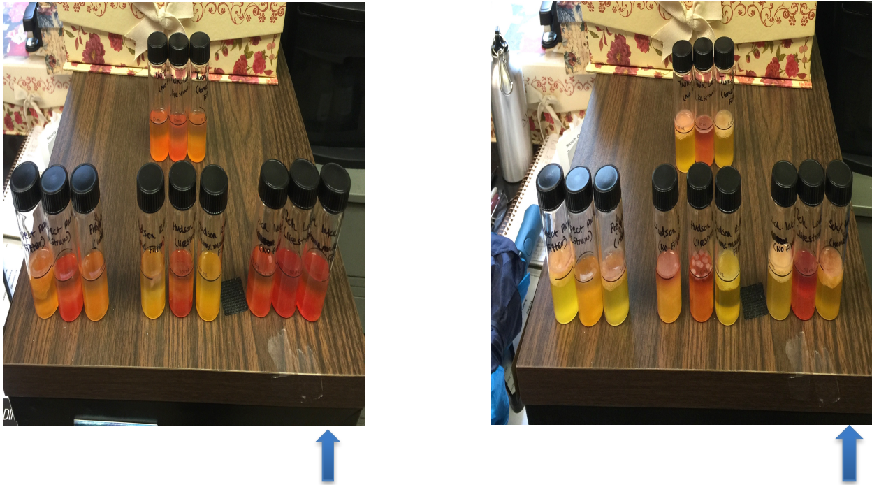
Figure 1. Results from coliform tests (Group 1) in which a simple plus/minus coliform test that works through a pH change if coliform bacteria are present. The samples change from red to yellow if coliform are present. Generally, the LifeStraw filtered better than the other filters the students devised.
