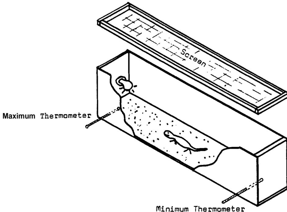
Figure 1. The photothermal gradient box. 1" deep sand on floor.
