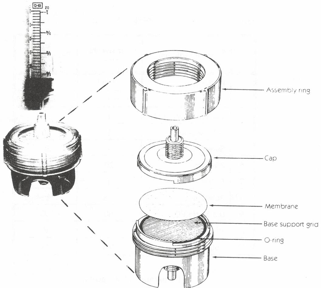
**Figure 8.5.** Schematic diagram of filtration assembly used to homogenize cells of *D. discoideum*.
