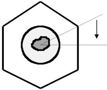
**Figure 9.2.** Demonstration of a 1/12<sup>th</sup> turn on the Nut-and-Bolt Microtome
