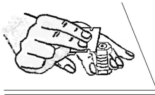
**Figure 9.1.** Correct hand position for use of the Nut-and-Bolt Microtome
