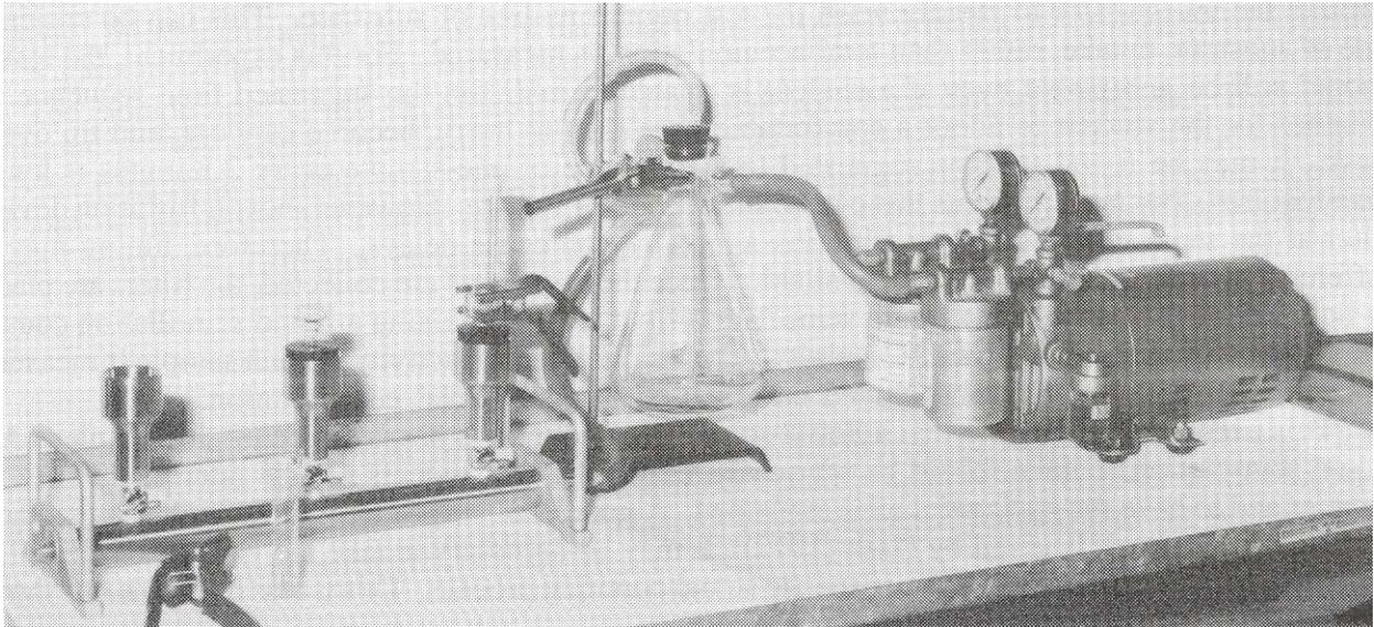
**Figure.9.3.** A workstation suitable for a pair of student is a vacuum manifold with filter units, a filtrate trap, and a vacuum pump; these are standing on absorbent paper in a tray that has a raised edge.
