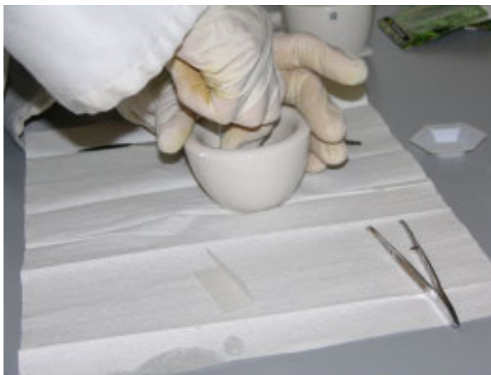
Figure 1. Seed preparation. After weighing, seeds are ground up with a mortar and pestle.
