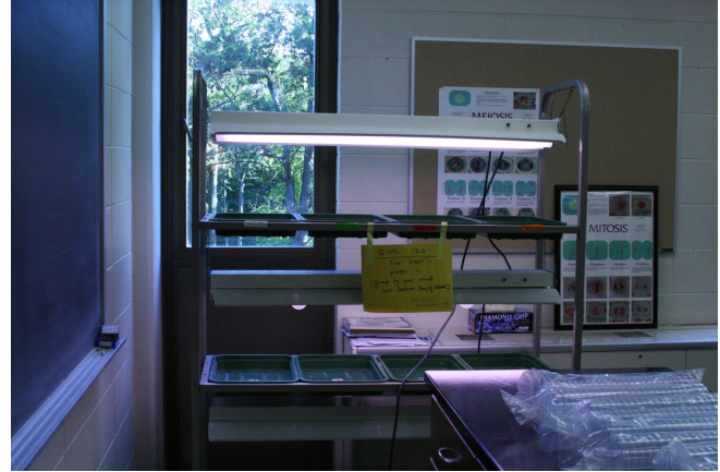
Figure 1. Light apparatus setup for 24-hour illumination of trays containing Petri dishes.
