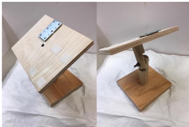
Figure 5. Assembled stand for solar panel support platform. Adhesive-backed hook and loop tabs attached to the upper support platform permit the small solar panel to be securely attached to the platform but easily removed after each use (Figure 7). A pyranometer sensor also may be attached to the support platform with adhesive-backed hook and loop tabs. Applying several coats of varnish to the wood prior to adding metal hardware and hook and loop tabs is optional.
