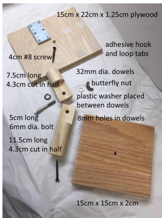
Figure 6. The disassembled solar panel support platform. The steel plate attached to the plywood panel is a steel mending brace 6.5cm x 3.5cm that will permit a magnetic angle locator to attach to the support platform. This steel plate could be attached to the platform with adhesive-backed hook and loop tabs rather than screwed to the plywood. The holes in both the plywood platform and the wood base are countersunk and wood screws pass through those holes to attach to the wood dowels.
